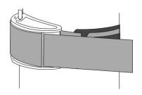
8. Clamp the cam buckle in position by pulling the end of the webbing.
