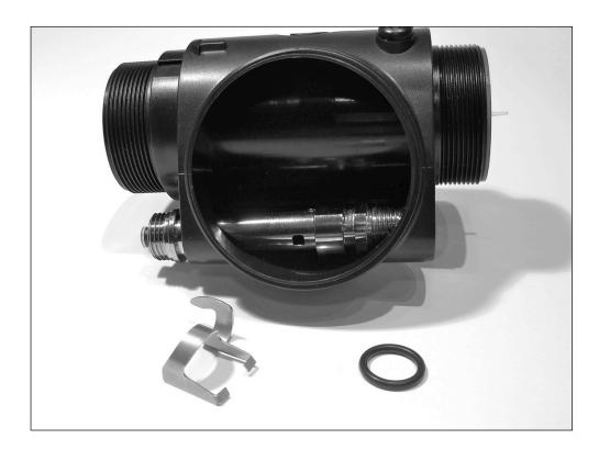
The picture above shows the removed lever, as well as one of holes in the steel tube
