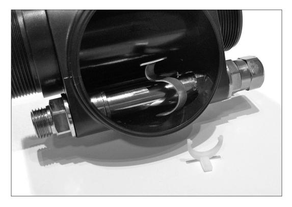
• Make sure you do <u>NOT</u> damage the small location cams on the curved part of the locking lever. They have an important role in fixing the locking lever into its position.
