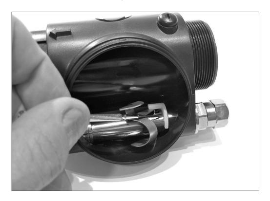
Gently pry the locking lever out of its position, using a very small screwdriver (e.g. a watch repair screwdriver as shown in the picture).
