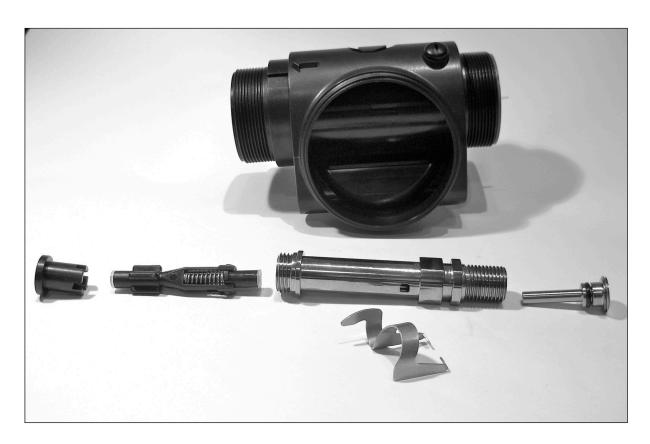
Next remove the steel tube from the main housing.
