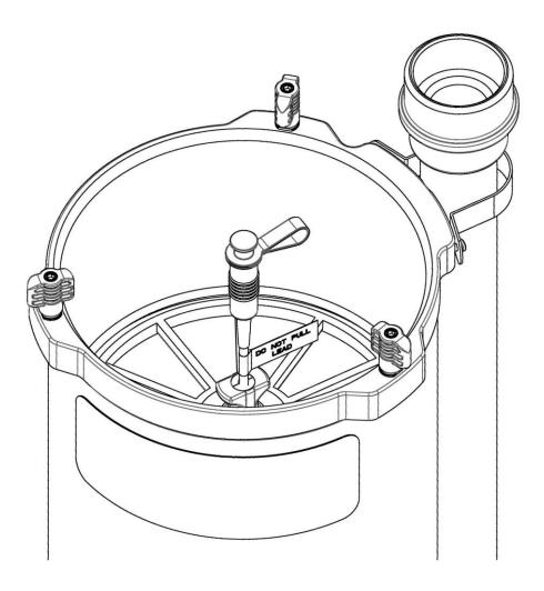
5. Assemble the lid into the canister and complete the rebreather setup as normal including all the pre-dive checks.
