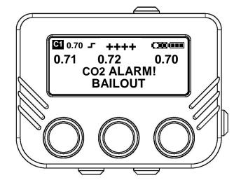
The CO<sub>2</sub> Sensor will trigger an alarm when CO<sub>2</sub> reaches 10 mbar in the breathing loop. The display will show "CO<sub>2</sub> ALARM! BAILOUT". This will cycle with any other warnings that might be present. The warning will also be shown on the Vision HUD, whilst the buzzer sounds. The HUD will show solid red lights on both controllers for the period that the CO<sub>2</sub> is above 5mbar.
