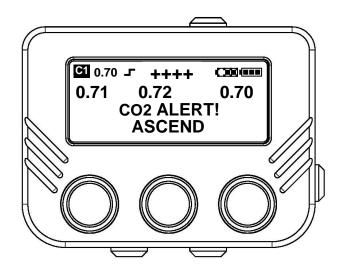
The CO<sub>2</sub> Sensor will trigger an alarm when CO<sub>2</sub> reaches 5mbar in the breathing loop. The display will show "CO<sub>2</sub> ALERT! ASCEND". This will cycle with any other warnings that might be present. The warning will also be shown on the Vision HUD, whilst the buzzer sounds. The HUD will show solid red lights on both controllers for the period that the CO<sub>2</sub> is above 5mbar.
