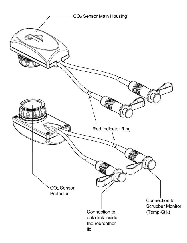
Note: A second Red Indicator Ring is supplied, which can be fitted to the Temp-Stik connector. This gives a quick visual indication as to which cables should be mated.
